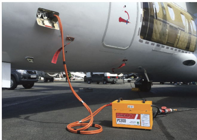
PS300: in operation on a Dornier 328
