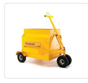
Transformer rectifier units (TRUs) delivering 600 amps continuous power – with the ability to briefly produce up to 1800 amps for engine starting – require a mains input of at least 63 amps (44Kw @ 400V) to accommodate the overload without tripping the supply circuit breaker. If there is insufficient power, upgrading the mains supply to handle the inrush current can be prohibitively expensive.
