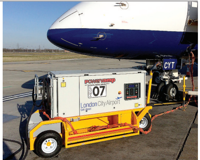
PV90-3: in operation at London City Airport
