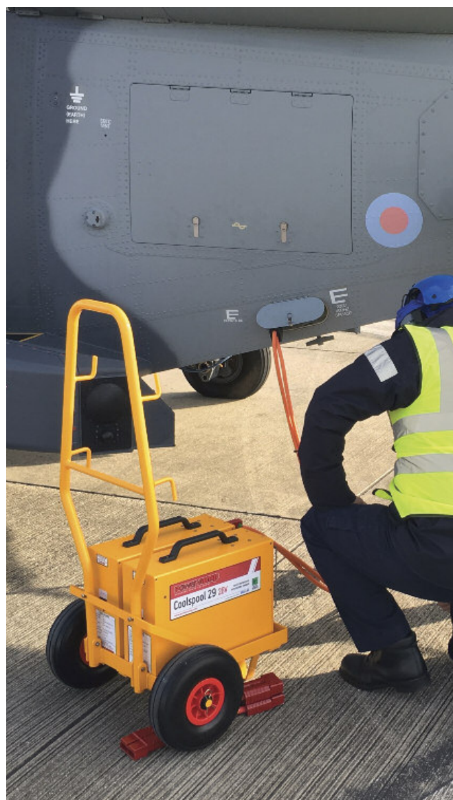
Coolspool 29 Twin: in operation with Lynx Wildcat
