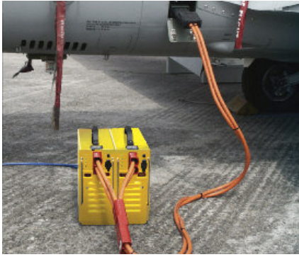
2 x PS100 in parallel: delivering up to 200 amps
