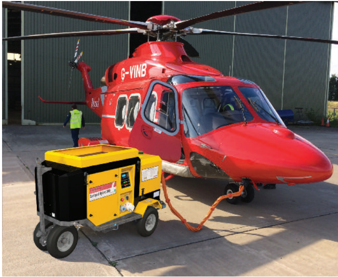
Coolspool Hybrid 300: starting both turbines on the Agusta Westland AW139
