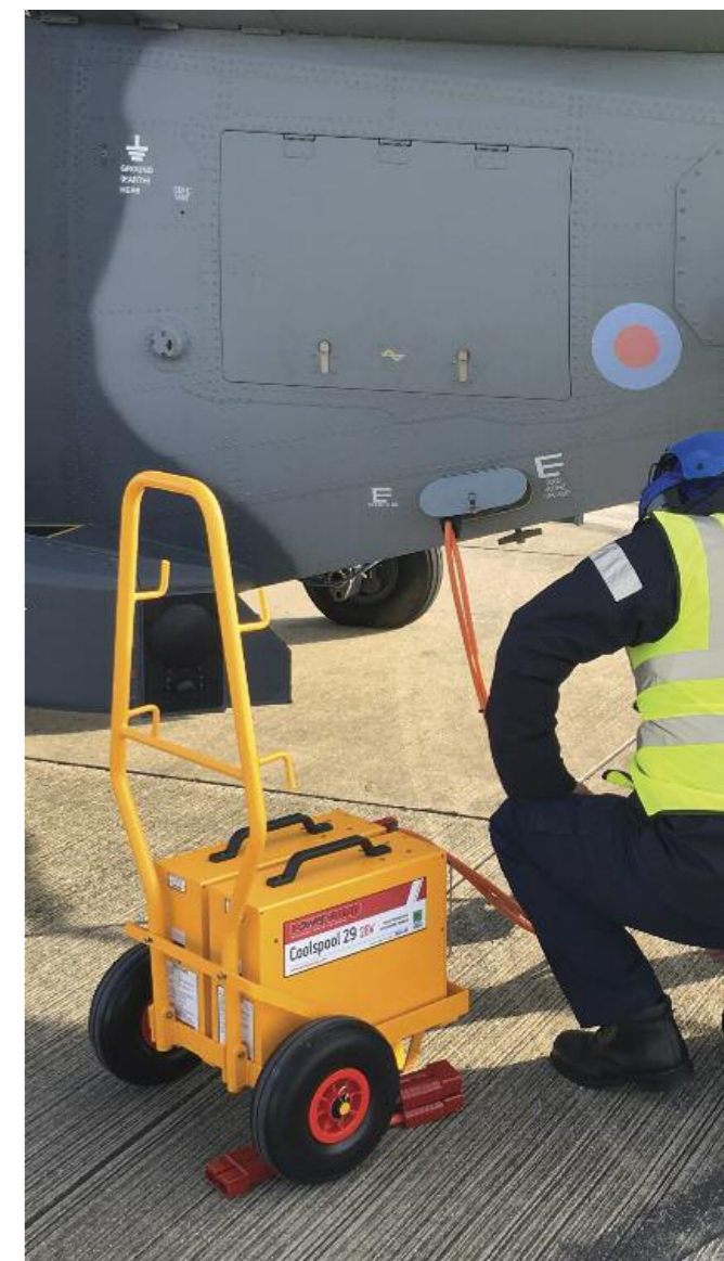
Coolspool 29 Twin: in operation with Lynx Wildcat
