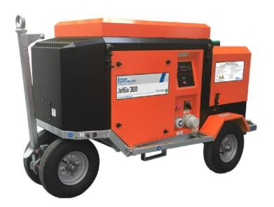
Available in various configurations and in series production over 17 years, with sales to several armed forces, the JetGo 300 is the civil version of Powervamp's DC GPU. It is designed for operators requiring versatile, standalone, high output DC power at a fraction of the cost of a conventional diesel GPU.
